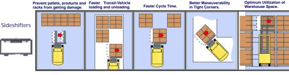
Use of Sideshifters permits the operator to shift the forks sideways instead of moving the complete fork lift, this ensures faster operation, better maneuverability in tight corners and optimum utilization of warehouse space permitting better storage density, resulting in well aligned stacking for efficient storage/retrieval and increase productivity.
